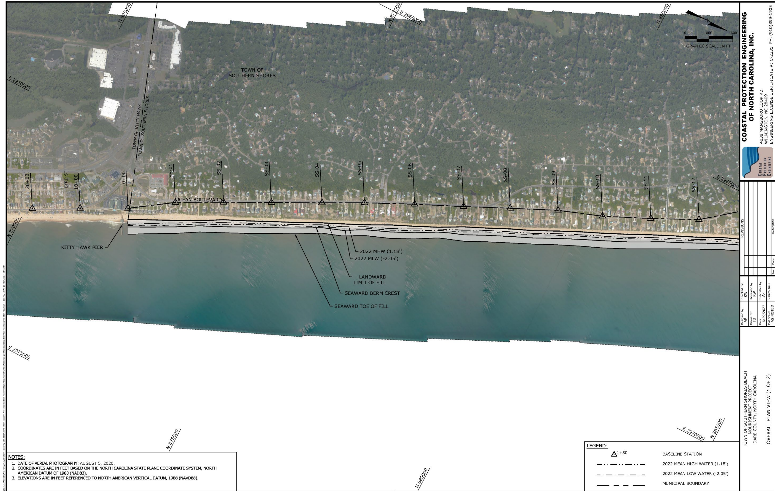
Figure 3. Map showing the extent of the 2022/2023 project including the main fill construction template and the construction baseline (1/2).
