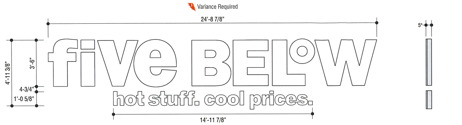
1 1 42" Channel Letters w/ Tagline - FB-FB42-TAG-IL-LNR-W-RM 122.4 sf Scale: 1/4" = 1' 0" (1 Required)
