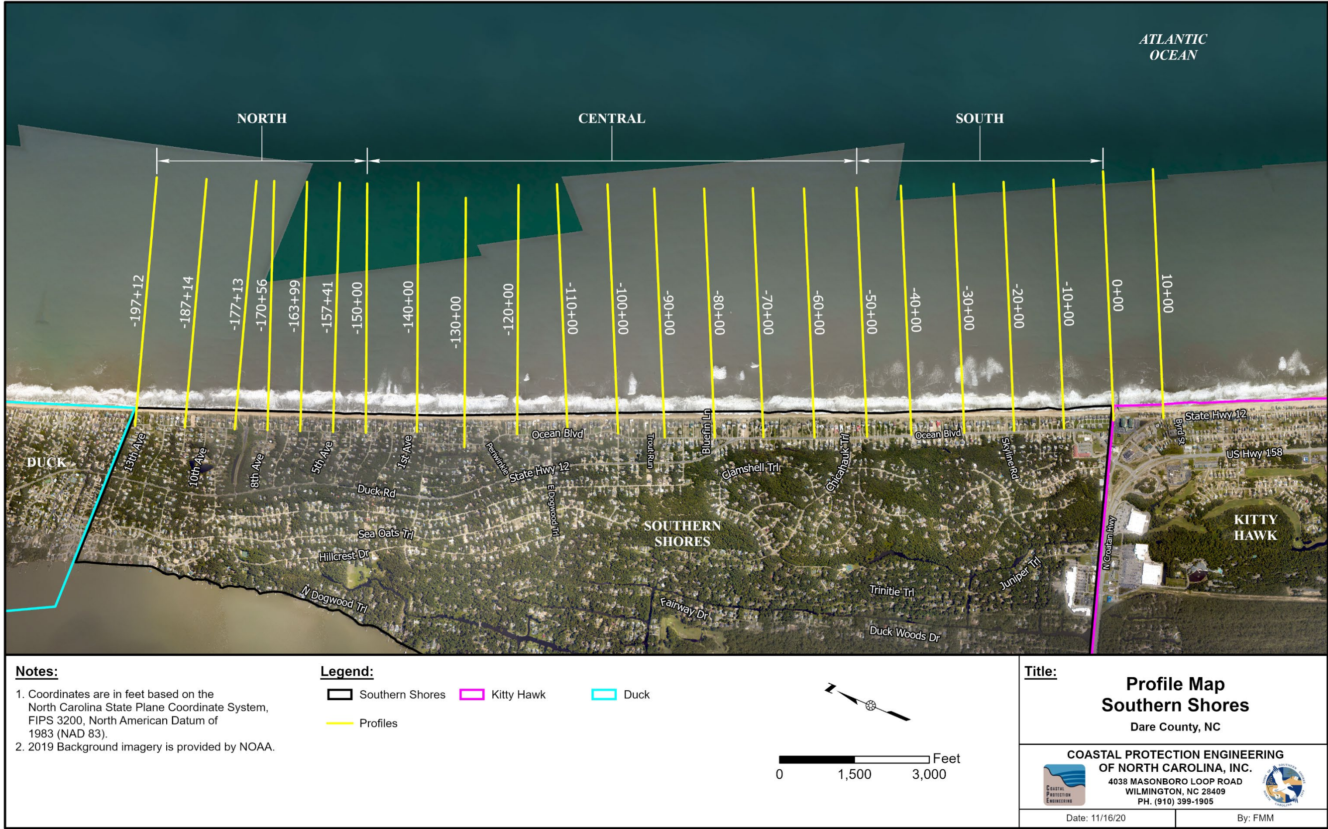
Figure 2. Map showing the location of the beach profiles along the Town of Southern Shores.
