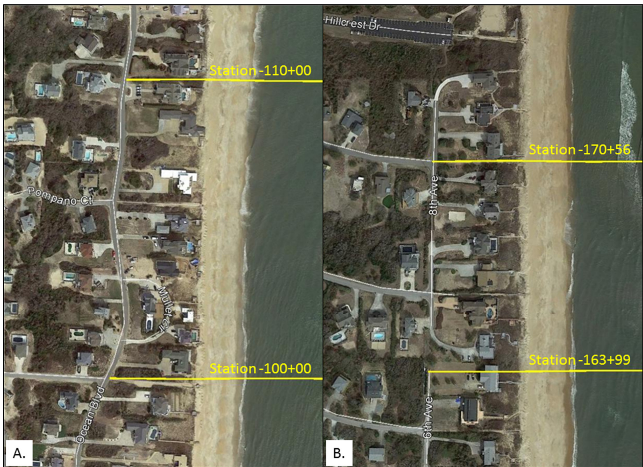
Figure 17. Google Earth Images from March 2017 showing the relatively minimal setback of structures from the vegetation between Stations -110+00 and -100+00 (A.) and the relatively greater setback of structures from the vegetation between Stations -170+56 and -163+99.
