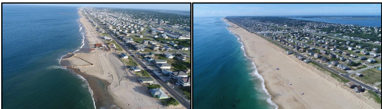
Figure 9. View of the beach nourishment project within the Town of Kill Devil Hills, looking south - Pre-Construction (left), Post-Construction (right).
